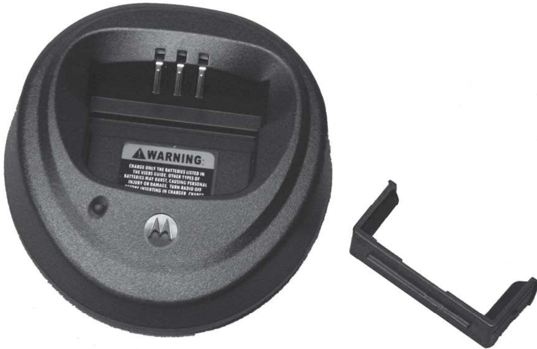
Figure 2 Battery Locating Rail removed
